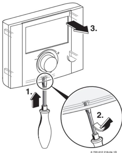
Fig. 2 Remove front casing
