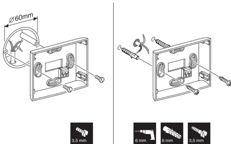
*Fig. 3 Fasten base plate to the wall*
